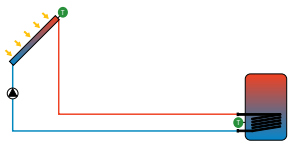
Internal heat exchanger, intelligent pump control
