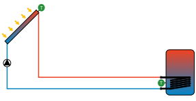
Internal heat exchanger, intelligent pump control
