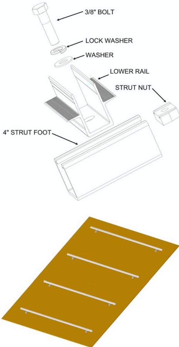
The lower rail is designed to be attached to SolarStrut™ feet or runners with a sliding strut nut assembly. The sliding strut nut assembly allows for fine adjustment on the spacing between adjacent lower rails.
