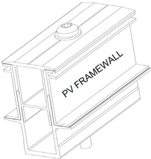
Most PV racking systems on the market today utilize dual strut style runners underneath rows of PV modules. Top-side clips are then used to attach the PV modules to the runners.
