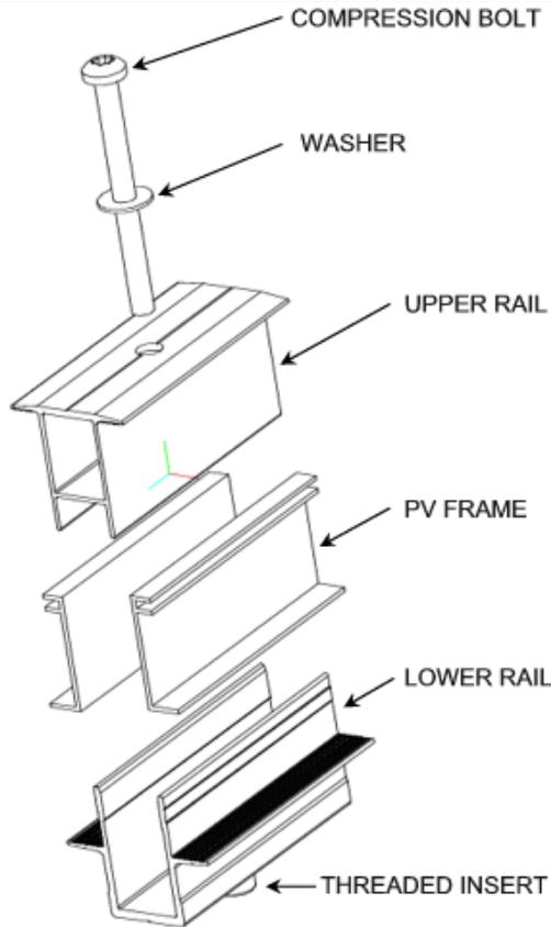
The CompRail™ system has two distinct components: an upper rail and a lower rail that are compressed by a 5/16"-18 stainless steel button head bolt. Both rails are fabricated from 6063-T6 aluminum alloy and are available in mill finish, clear or bronze anodized material.
