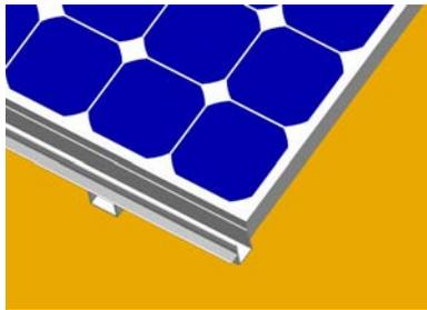
Once the lower rails have been set in place, lay the modules down between the rails with the module framework resting on the integral shelves.
