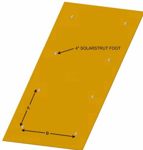
SolarStrut™ feet or runners must be attached to the roof to hold the lower CompRail™ in place. The figure at the left shows SunEarth 4" SolarStrut™ feet lagged to the structural members of the roof in a pattern that accommodates 3 vertical banks of modules.
