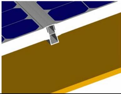
With the PV modules in place, the upper rails may be placed into the shared lower rails and bolted together.
