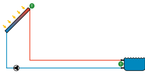
Direct flow-through, intelligent pump control
