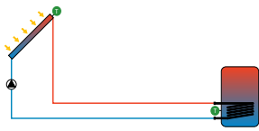
Internal heat exchanger, intelligent pump control
