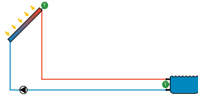
Direct flow-through, intelligent pump control
