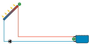
Direct flow-through, intelligent pump control
